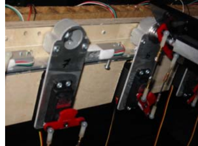
Fig. 9. Custom-made aluminum parts are attached to servo motors and load cells. Red plexiglas parts connect the servos with the planks.
